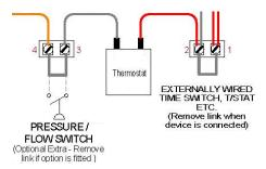
Where an external thermostat is utilised the water heater thermostat should be adjusted to a temperature higher than the setting on the remote thermostat (Refer to "Temperature Control" on page 35.
